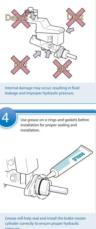
Do not allow dust, dirt, and debris to enter
