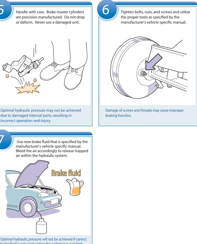
due to damaged internal parts, resulting in incorrect operation and injury.
