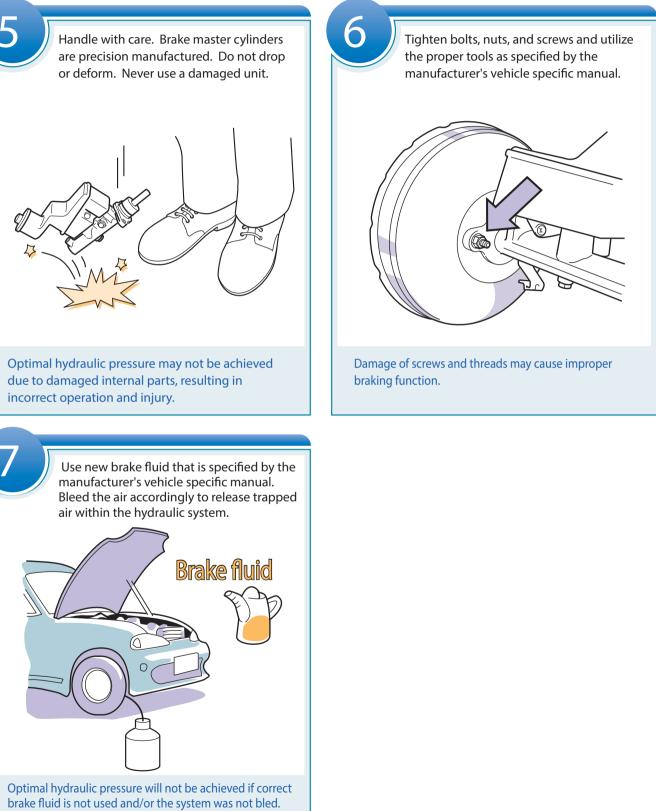
Brake failure may occur causing damage and injury.
