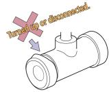
If the boot is not installed correctly, foreign objects could enter the mechanical assembly, causing insufficient brake control.
