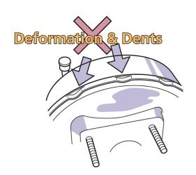
Insufficient pressure or leaks may occur if damaged.
