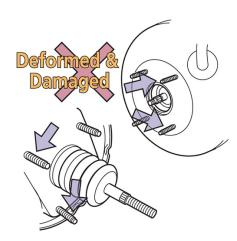
Brake booster may not mount properly causing failure to operate correctly.
