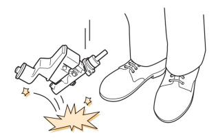
Internal parts may be damaged and the brake booster may fail to operate correctly.
