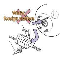
It could cause rust formation at the inside or damage seals so that the brake booster may fail to function properly. Failure to follow recommended procedures may cause brake failure and injury. Always consult the manufacturer's vehicle specific service manual for reference.
